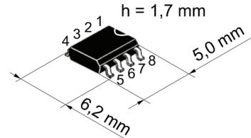
SO8 Housing (150 mil, Standard SMT Technology, SOIC-8) as per IEC 191-2Q: Type 076E35 B
