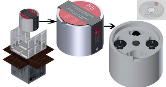
ATTENTION! The styrofoam packing is used for calibration. Please do not discard.
