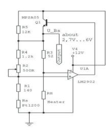
Both elements (Heater RH and sensor RS) can be switched in a bridge. The resistors R1,R2 and R3 determine the temperature difference ( $\Delta$ T) between RS and RH. This is the condition to which the voltage fitting to the bridge is controlled.
