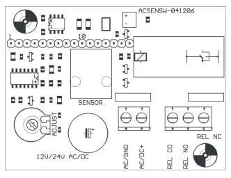
The RJ12-plug connector is provided for direct connection to the sensor switching module (SENSOR plug socket).
