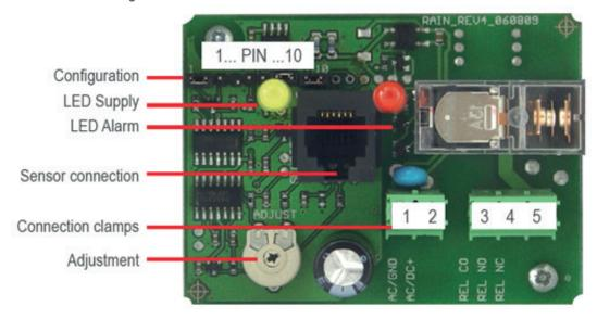
The RJ12-plug connector is provided for direct connection to the leakage detector (sensor connection).
