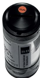
The humidity probe is supplied in calibrated condition. The accuracy at 23°C is of the order of  $\pm 0.3$  K and  $\pm 2$  % RH. Under normal operating conditions, it is not necessary to again calibrate the probe. The cross checking of measuring accuracy of the humidity measurement part can be done by end user with the salt reference cells available as special accessories.
