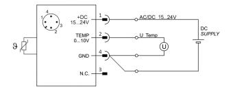
Humidity measurement 0  $\dots$  10 V und Temperature measurement 0  $\dots$  10 V
