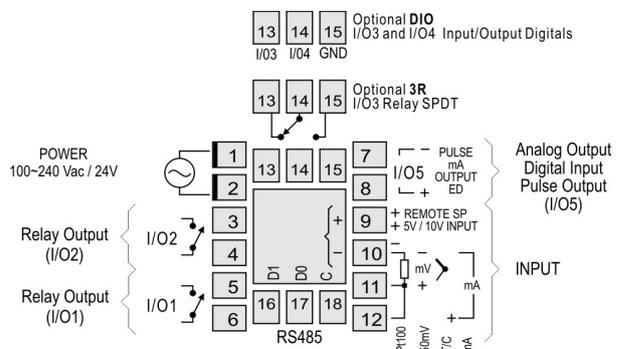
**Figure 1 - Connections of the back panel**
