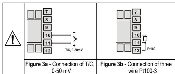
Figure 3a - Connection of T/C, 0-50 mV
