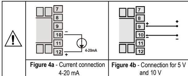
Figure 4a - Current connection 4-20 mA
