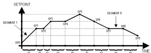
Figure 8 - Example of a Ramp and Roak.
