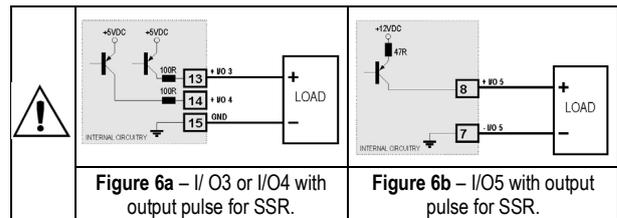
Figure 6a – I/O 3 or I/O 4 with output pulse for SSR.
