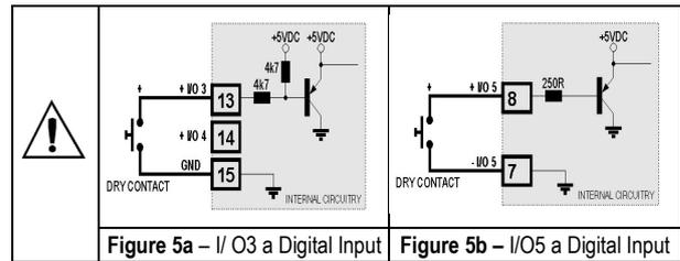
Figure 5a – I/O 3 a Digital Input
