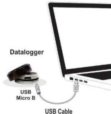
Fig. 04 – Communication via USB cable
