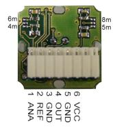
There are four soldered joints on the back side of the module. By closing (over-soldering) one of the jumpers, the sensitivity of the module can be reduced.
