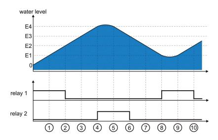
Initial condition: The reservoir is first empty. The electrode E1 is not in water contact. Relay 1 is in closed position (because of this e.g. the inlet valve is open). The water level rises in the reservoir. Water contact with the lower Electrode E1 (1) does not change the relay status and only when Electrode E2 comes into water contact (2), Relay 1 switches OFF (as an effect e.g. the inlet valve closes).
