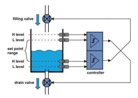
In liquid reservoir, four electrodes (E1..E4) are mounted in the medium, at heights corresponding to the required switching point. A fifth electrode is placed at the bottom of the reservoir (not shown in sketch) which works as the reference electrode.
