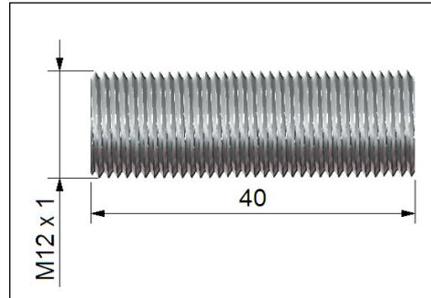
The sighting tubes can only be used for sensing heads with a distance-to-spot ratio (D:S) of  $\geq 15:1$ .
