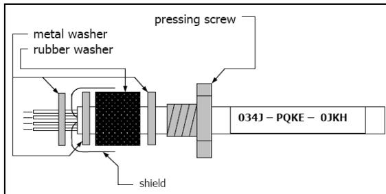
Use shielded cables only. The sensor shield has to be grounded.
