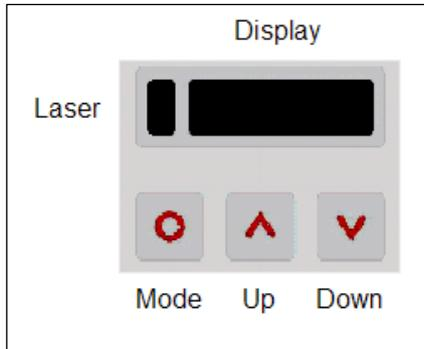
Pressing the Mode button again recalls the last called function on the display. The signal processing features **Peak hold** and **Valley hold** cannot be selected simultaneously.
