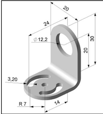
Mounting bracket, adjustable in one axis
