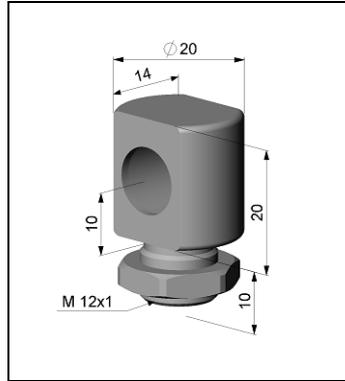
Mounting bolt with M12 x 1 thread, adjustable in one axis
