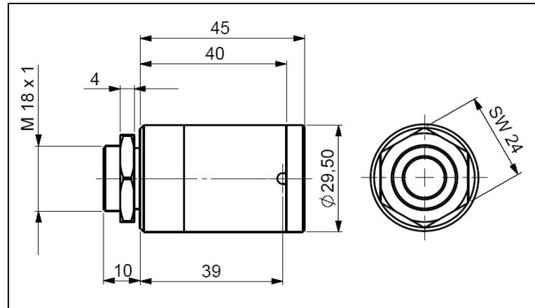
Massive housing (Standard on DM-Hot and P7)
