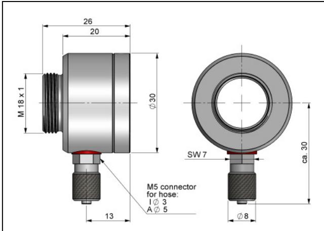
Air purge collar for massive housing (thread M18 x 1)
