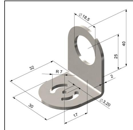
Mounting bracket for massive housing,
