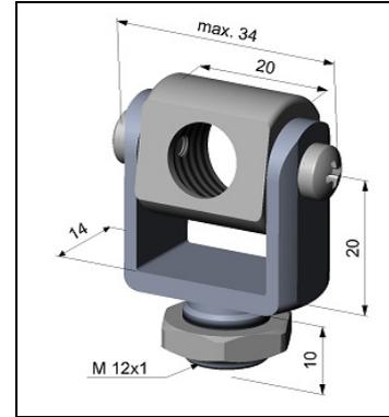
Mounting fork with M12 x 1 thread, adjustable in 2 axes
