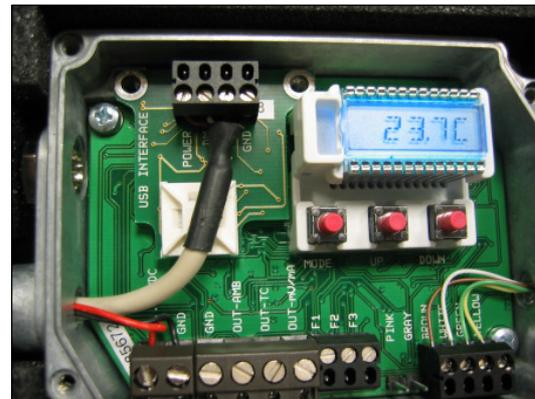
The switching thresholds are in accordance with the values for alarm 1 and 2 [► Alarms/ Visual Alarms]. The alarm values are set according to the ► Factory Default Settings. To make advanced settings (change of low- and high alarm) a digital interface (USB, RS232) and the software is needed.
