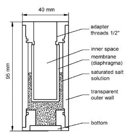
The cells have a mechanically stable and leak-proof construction. The inner wall forms a membrane (also referred to as the diaphragm) which separates the test chamber from the salt solution. The diaphragm is a micro-porous, water vapour permeable wall, which restricts contact of test objects with the salt solution. The sealing is also effective for a short time use in "overhead".
